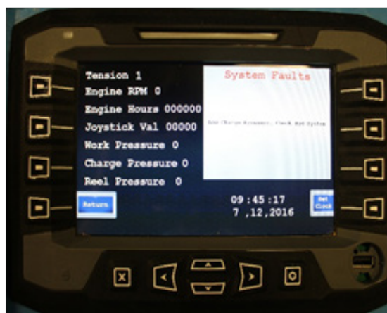
FIGURE 17: System Faults Alert
