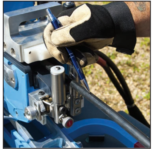
Figure 14. Mark the Cable
