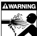
**!WARNING:** Forced air creates flying debris. Always wear personal protective equipment. Severe personal injury could result.
