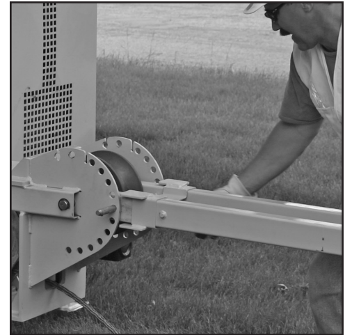
Figure 3. Lock Boom in Place
