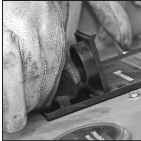
Figure 7. Turn Ignition Key while Holding Rocker Switch
