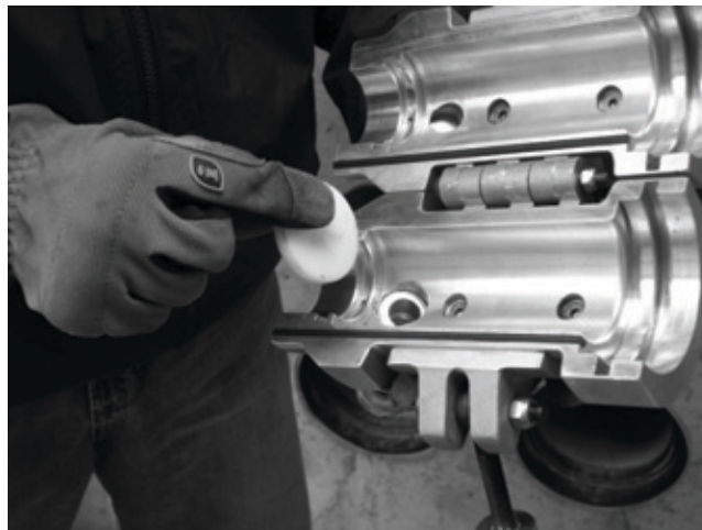
Figure 2 Insert Seal Disk Plug
