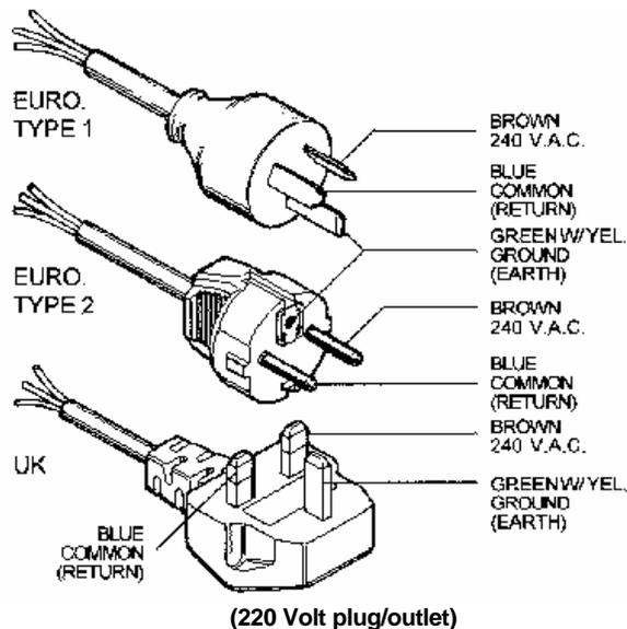
Figure 2 Properly grounded plug/outlet connections
